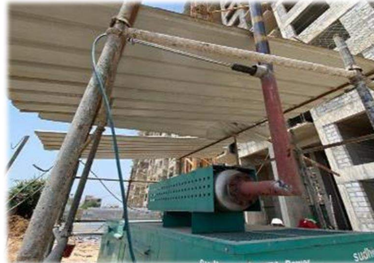
Measuring exhaust emission
